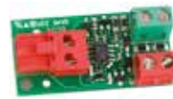
BUS XIB interface (for E045 or E045S or E024S boards with photocell no BUS)
